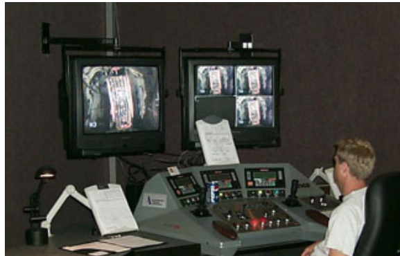
Figure 52: Teleoperation of a drill at the Stobie mine using video and joysticks.
