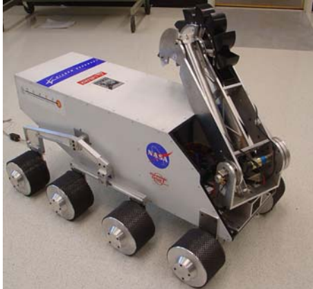
Figure 10: The CSM's Lunar Bucket Wheel Excavator concept vehicle
