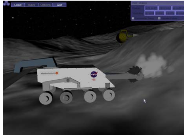
Figure 24: BWE bucket wheel "biting in" with simulation of dust effects.
