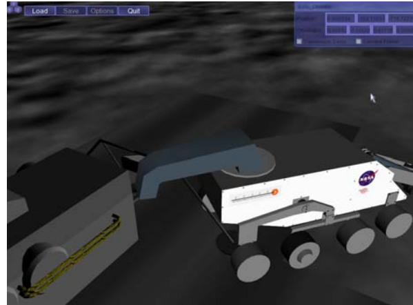
Figure 28: BWE off normal and colliding with support stand for ISRU processor.
