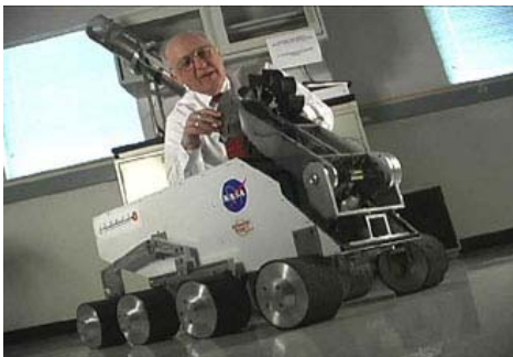
Figure 2: Dr. Michael Duke with Colorado School of Mines' Lunar Bucket Wheel Excavator (R. King, T. Muff, M. Duke).
