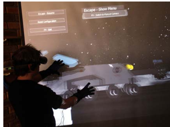
Figure 18: BWE on autostereo display on which both left and right display frames are synchronized with shutter glasses for depth.
