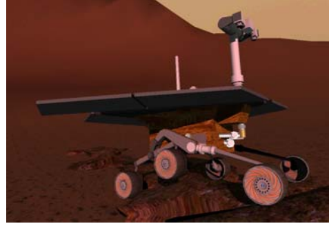
Figure 49: DigitalSpace's physics-based real-time model of the MER vehicle
