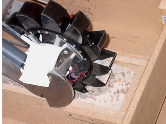
Figure 11: Bucket wheel operating in testbed simulant
