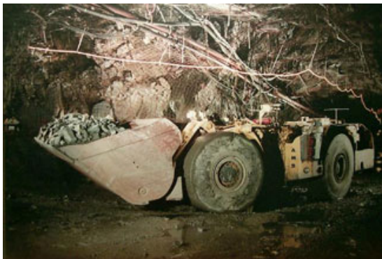
Figure 51: Automated excavator at INCO's Stobie mine in Canada.
