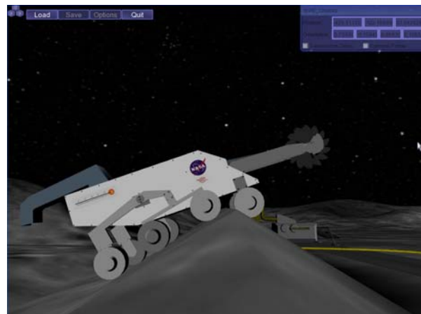
Figure 26: BWE caught on hilltop showing physics action of double rocker-bogie mechanism. Vehicle is able to back out.
