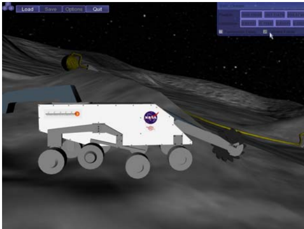
Figure 23: BWE in drive mode over simulated regolith.
