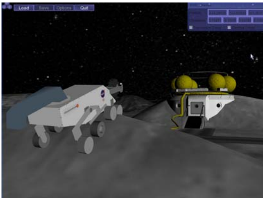
Figure 19: the BWE scaling a landing exhaust berm to habitat in analogue lunar base
