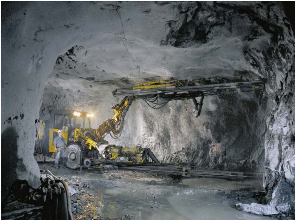
Fig 28: Atlas Copco drill jumbo at work in mine
